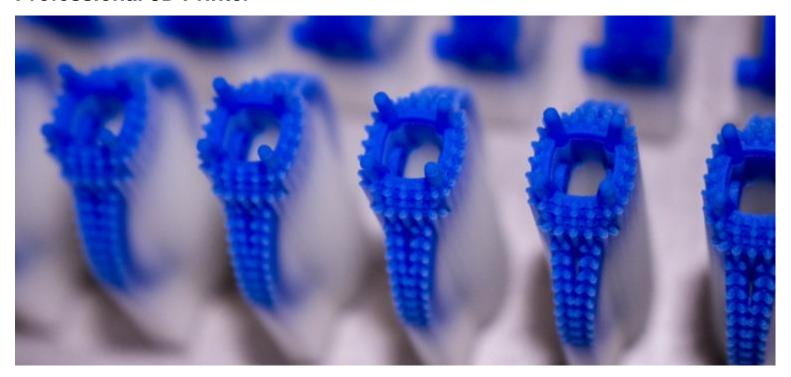
The ProJet MJP 3600W produces mirror standard wax casting patterns with outstanding precision and micro-detail. An expanded print envelope increases total throughput and accommodates larger-sized parts.
