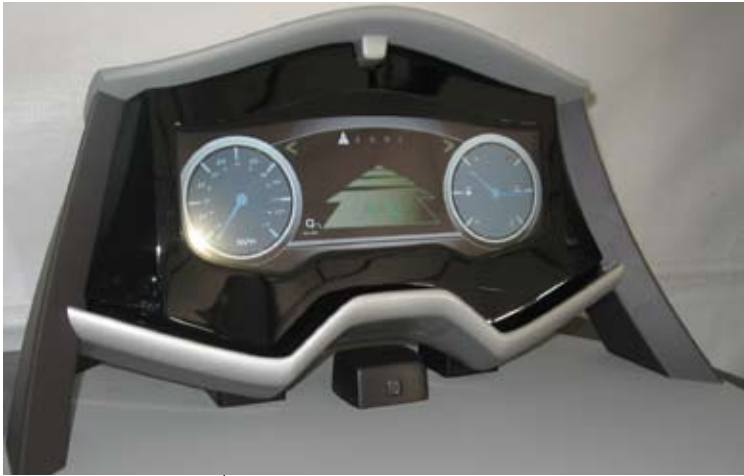
The automotive cluster concept was constructed from several ZPrinter printed parts.
