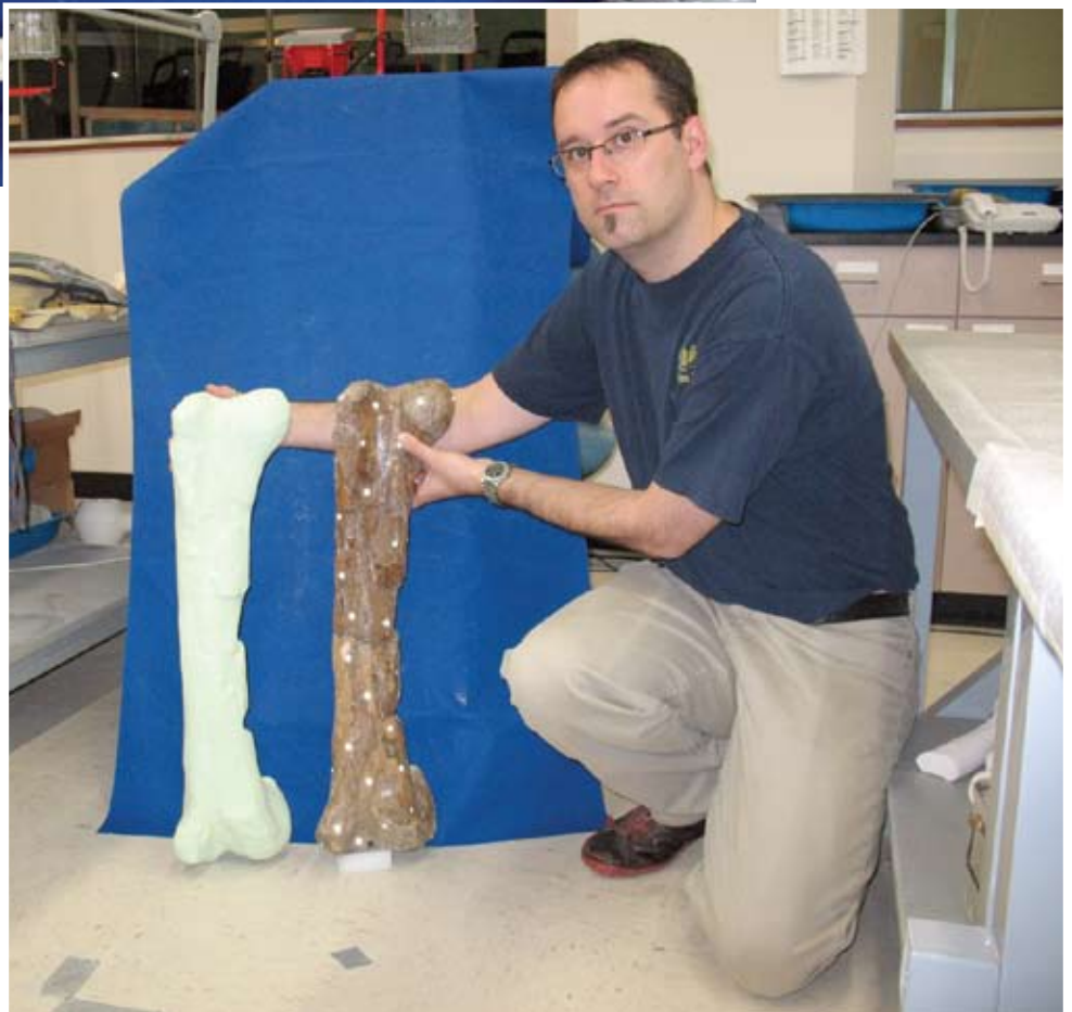
A technician holds up an actual bone with reflective targets (right) and the printed results.
