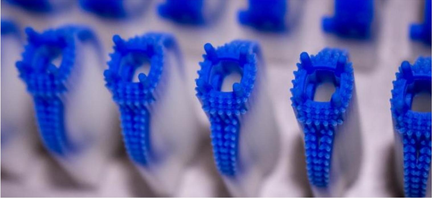
The ProJet MJP 3600W produces mirror standard wax casting patterns with outstanding precision and micro-detail. An expanded print envelope increases total throughput and accommodates larger-sized parts.
