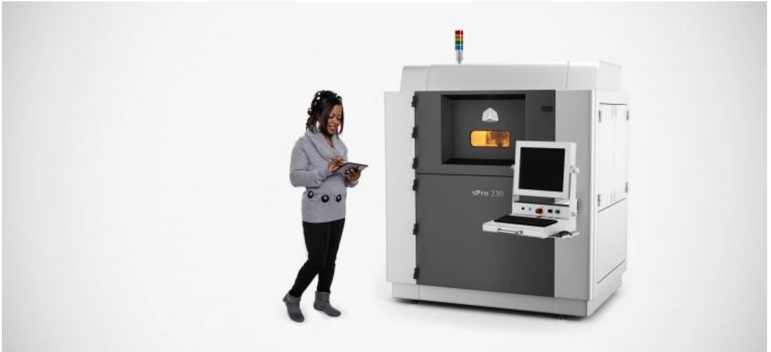
The sPro 230 production printer uses a state-of-the-art digital imaging system to accurately build large (up to 30 in/750 mm long), durable plastic parts in high-definition. Profit from the fullest use of the broadest range of available materials with automated powder handling and material recycling and traceability.
